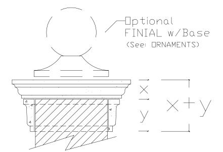
Wall Cap and Pier Cap Profiles (X) may be enhanced by the placing of an additional moulding (Y) below the expanded cap.
